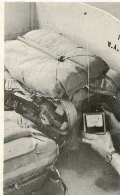
Pin-pointing a chute with a malfunctioning beeper is simple with NASA's signal detector. When the general location is determined, detector sensitivity is reduced (left). Meter reading increases (right) as snooper nears the beeping chute.
