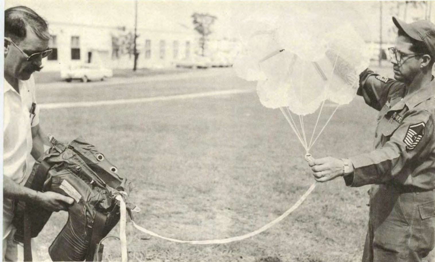
When manually actuated the parachute is pulled out by a small pilot chute instead of the five foot drogue.
